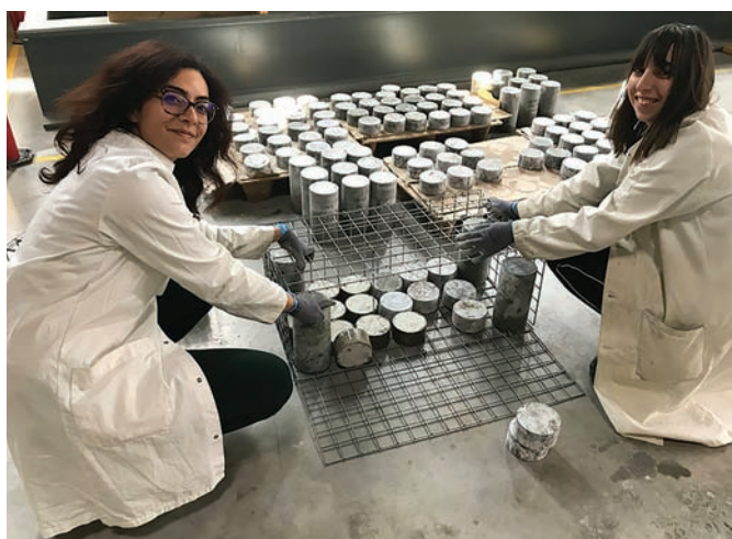
ESITC Caen PhD student Marine Georges and researcher Amel Bourguiba with concrete samples to be deployed in Dinard bay, France
