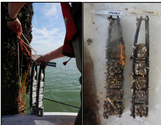
Concrete sample tiles and oyster shell control deployed for testing biological colonisation
