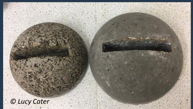
Two concrete mixes being trialled for crevice units.
