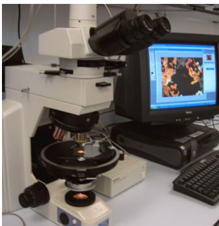
Left: A petrographic microscope. Right: A QEMSCAN ®
