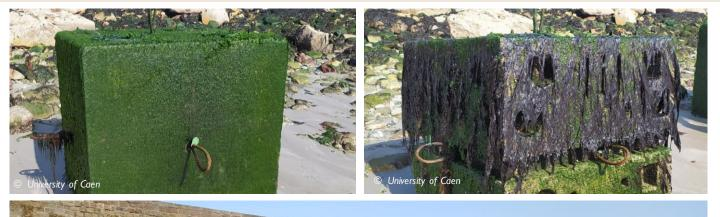
Top: a plain breakwater module (left) covered in green seaweed and an experimental breakwater module covered in a variety of green and red seaweeds. Bottom: the breakwater modules on the shore at Cherbourg Harbour, France. Inset: the concrete cylinders for durability testing.
