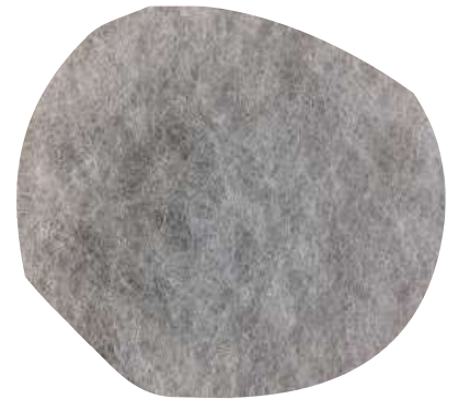
geotextile NW170 White non-woven (170 g/m2)
